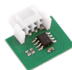
P-250SM120 Memory card for 120 radio codes
