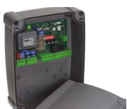
P-750D770M Electronic control unit for one or two 230 V gate operators with soft-stop and built-in 433,92 MHz rolling code radio receiver, complete with enclosure
