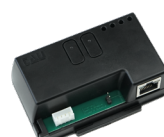
P-250T-CONNECT Ethernet + Wi-Fi device - to enable through Tau Open 2.0 application, the use of the smartphone remotely, to open/ close and check the status of the gate
