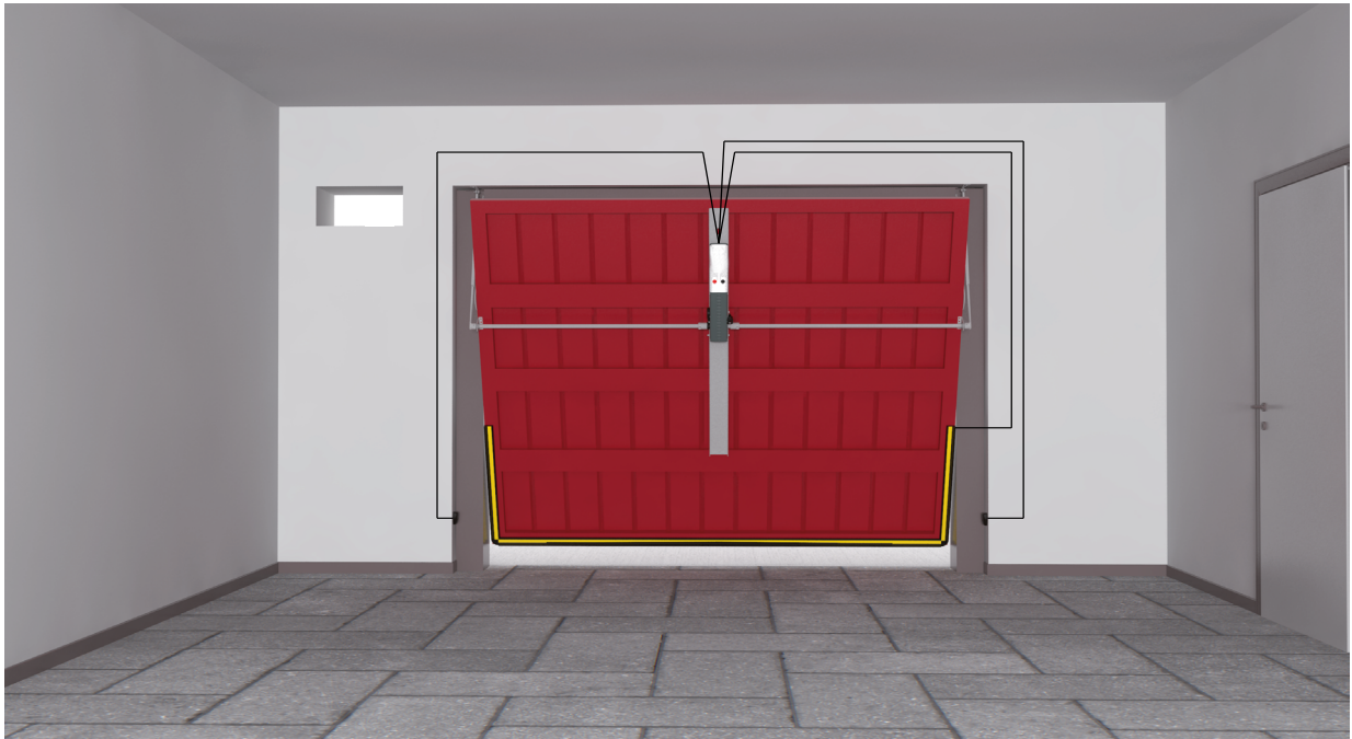
TYPICAL SYSTEM WITH CENTRAL MOUNTING
