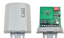
P-900TWM Master receiver for central interface (manages up to max. 4 TWCs)
